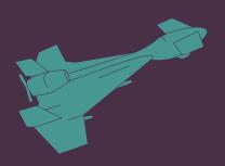
This 2.1m long 'loitering' missile is launched from a ground vehicle. It is armed with a 15 kg explosive warhead. The Harpy can loiter for up to 9 hours at a time, searching for enemy radar signals. It automatically detects, attacks and destroys enemy radar emitters by flying into the target and detonating.
