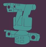
This stationary robot, armed with a machine gun and a grenade launcher, operated along the border between North and South Korea. It can detect human beings using infra-red sensors and pattern recognition software. The robot has both a supervised and unsupervised mode available. It can identify and track intruders, with the possibility of firing at them.
