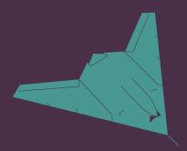
This 10m long stealth unmanned combat aircraft can fly autonomously for over 3 hours for autonomous detection, localization, and reconnaissance of ground targets. The Neuron has fully automated attack capabilities, target adjustment, and communication between systems.
