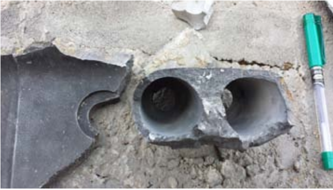
Remnants of a US-made GBU-12 Paveway II laser-guided bomb recovered at the scene of the wedding attack. Pen shown for scale.
