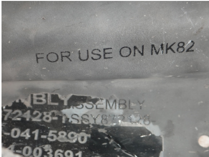
Remnant of a US-made GBU-12 Paveway II bomb used in an attack on a civilian home in Dar Sa'ad District, Aden Governorate (see Section II). As the marking "FOR USE ON MK82" indicates, an Mk-82 warhead was mounted on the GBU-12 bomb. The marking "1325-01-041-5890," parts of which are visible in the photo, is associated with a Raytheon-manufactured wing assembly.
