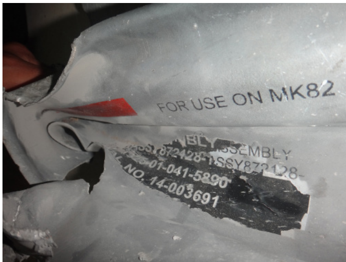
Remnants of a US-made GBU-12 Paveway II bomb recovered at the scene of the attack that killed Haifa Zawqari. As the marking “FOR USE ON MK82” indicates, an Mk-82 warhead was mounted on the GBU-12 bomb. The marking “1325-01-041-5890,” parts of which are visible in the photo on the left, is associated with a Raytheon-manufactured wing assembly.
