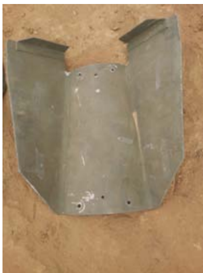
A remnant of a likely US-made CBU-58 cluster bomb used in the attack on Mohammed Saheli’s farm. The remnant pictured appears to be a tail unit of the bomb. The CBU-58 cluster bomb disperses about 650 BLU-63 submunitions widely and indiscriminately.
