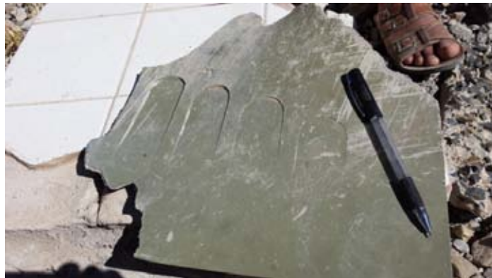
Remnants of a likely US-made GBU-24 Paveway III laser-guided bomb found at the scene of the attack on the Wa'lan Agricultural Complex. The photo on the right appears to show the forward fin of a guided bomb unit. The parallel indents with circular ends match the configuration of the GBU-24. The photo on the left appears to show the tail wing of a guided bomb unit. The two indents match the configuration of the GBU-24.
