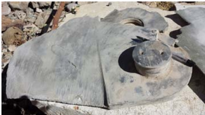
Remnants of a likely US-made GBU-24 Paveway III laser-guided bomb found at the scene of the attack on the Wa'lan Agricultural Complex. The photo on the right appears to show the forward fin of a guided bomb unit. The parallel indents with circular ends match the configuration of the GBU-24. The photo on the left appears to show the tail wing of a guided bomb unit. The two indents match the configuration of the GBU-24.
