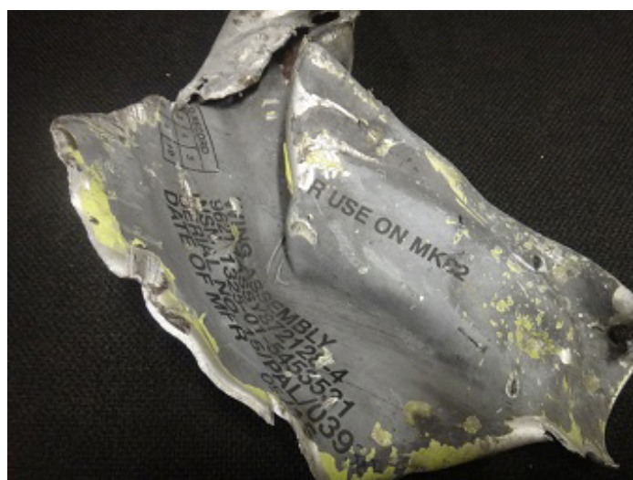
Remnant of a UK-made Paveway IV bomb found at the scene of the attack on Al-Muqbeli Warehouse. As the marking “FOR USE ON MK-82” indicates, a US-made Mk-82 warhead was used with the Paveway IV bomb. The marking “NSN1325-01-545351” is associated with the Paveway IV wing assembly. The marking “96214” identifies Raytheon as the manufacturer, and the marking “05/15” identifies the weapon’s date of manufacture as May 2015.
