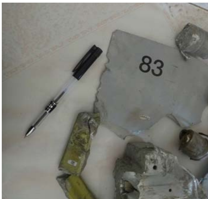
Remnants of a US-made Mk-83 warhead found at the scene of the attack on Al-Kahlani Factory. The Mk-83 warhead is associated with the GBU-16 Paveway II bomb. Left: The marking "8,000 PSI" is consistent with the gas containers of a number of GBU forward control units, which are pressurized to 8,000 PSI. The marking "252746-5" is associated with Raytheon aircraft parts.
