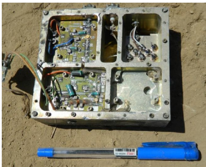
Remnants of a UK-made “Hakim” A series precision guided munition (PGM) found at the scene of the attack on the community college. The markings on the remnant in the photo on the right identify GEC-Marconi Dynamics as the manufacturer.
