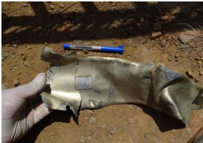
Remnants of a UK-made Paveway IV bomb found at the scene of the attack on Al-Senidar Factory Complex. As the remnant in the photo on the right indicates, a US-made Mk-82 warhead was mounted on the Paveway IV bomb. The marking “96214” on the remnant in the photo on the right identifies Raytheon as the manufacturer.
