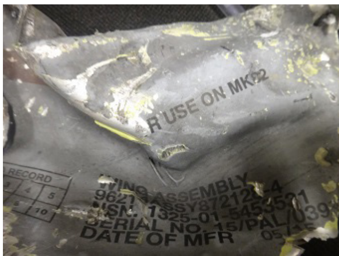
Remnant of a UK-made Paveway IV bomb found at the scene of the attack on Al-Muqbeli Warehouse. As the marking “FOR USE ON MK-82” indicates, a US-made Mk-82 warhead was used with the Paveway IV bomb. The marking “NSN1325-01-545351” is associated with the Paveway IV wing assembly. The marking “96214” identifies Raytheon as the manufacturer, and the marking “05/15” identifies the weapon’s date of manufacture as May 2015.
