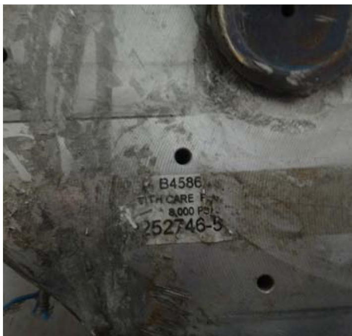
Remnants of a US-made Mk-83 warhead found at the scene of the attack on Al-Kahlani Factory. The Mk-83 warhead is associated with the GBU-16 Paveway II bomb. Left: The marking "8,000 PSI" is consistent with the gas containers of a number of GBU forward control units, which are pressurized to 8,000 PSI. The marking "252746-5" is associated with Raytheon aircraft parts.
