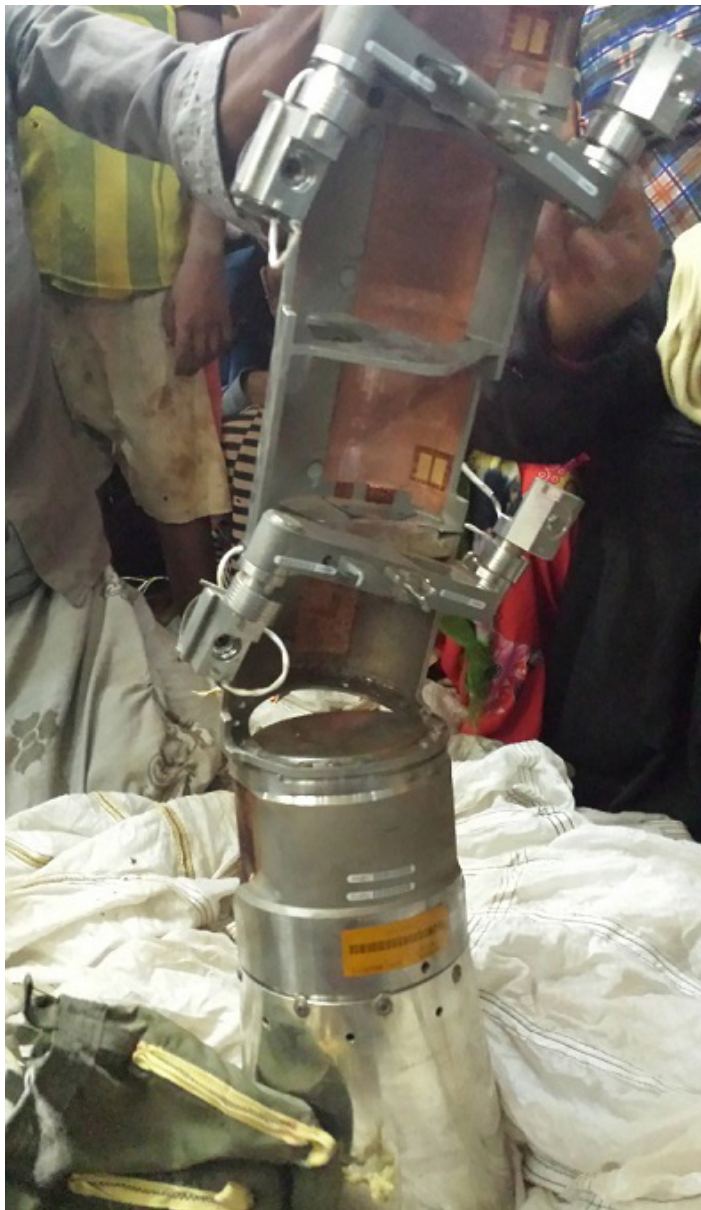
A stabilization unit of a BLU-108 submunition, recovered at the scene of the attack that killed Ali Mudarij. The marking “ASSY 856283,” visible in lower photo, is associated with the US-made CBU-105 cluster bomb, which releases BLU-108 submunitions. Each BLU-108 submunition contains four further “skeet” submunitions.
