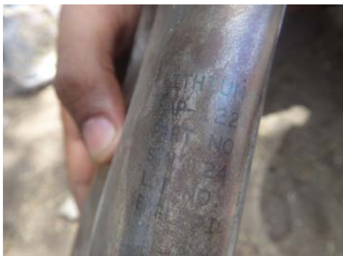
Remnants of what appear to be a US-made JDAM GBU-31 bomb found at the scene of the attack on Asma'a bint Abi Bakr School. Above: The four securing holes in the fin-shaped remnant in this photo resemble those of a JDAM GBU-31 tail fin. The silver item in the forefront of this photo may therefore be a JDAM GPS antenna. Below: The marking "LITHIUM" on the remnant in this photo is consistent with the JDAM tail actuator system, which contains a lithium battery.
