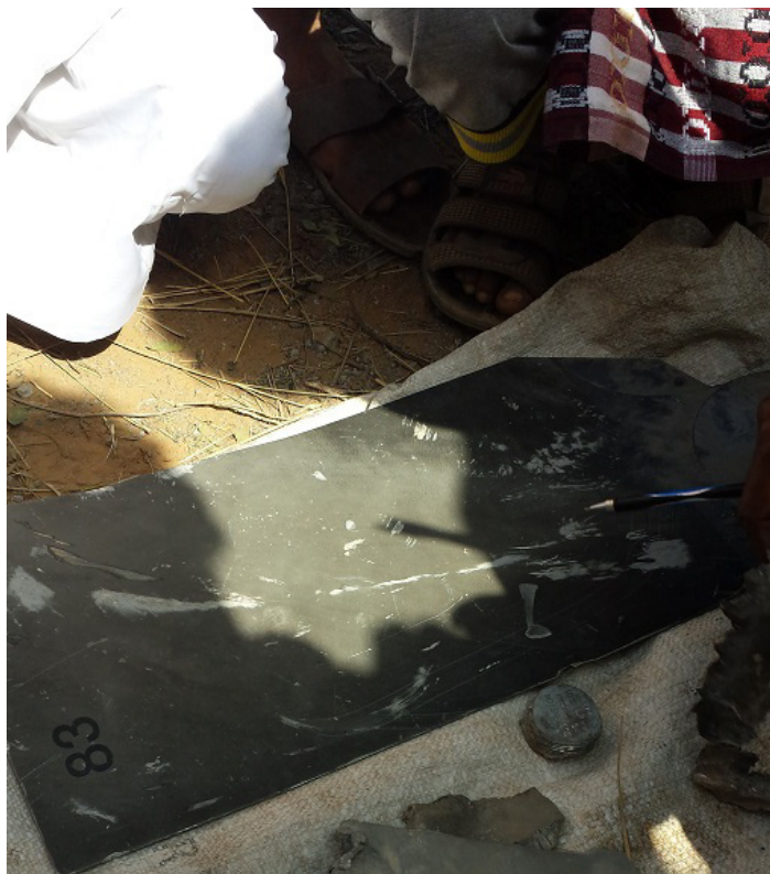
Remnants of a likely US-made GBU-16 bomb recovered at the scene of the attack in Dir Al Hajri village. The number 83 in the photo on the left appears to be associated with the Mk-83 warhead. The marking “MS3314” in the photo on the right is associated with 1000-pound bomb suspension lugs, which are consistent with the Mk-83.
