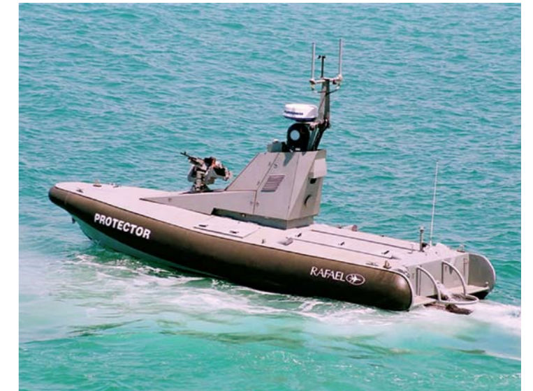
The armed USV 'Protector', in use with the navies of Singapore and Israel. © Rafael Advanced Defense Systems
