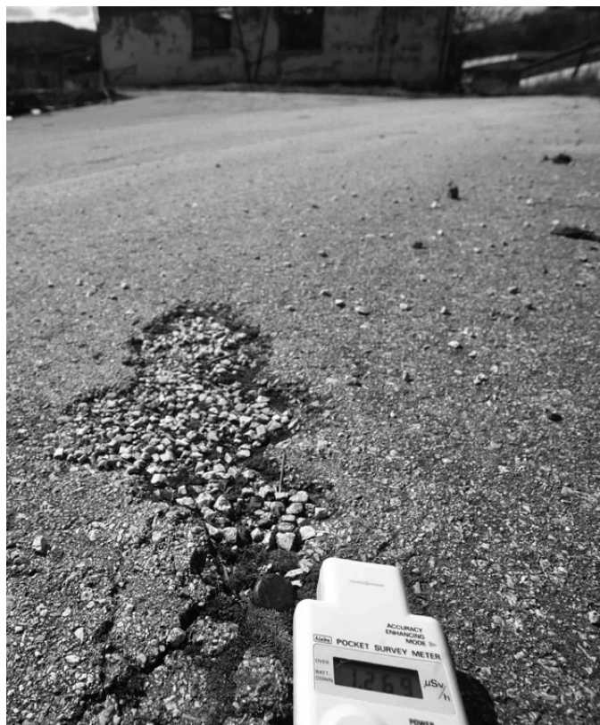
Steel peg marking impact hot spot on the tarmac apron at the TRZ facility, gamma reading is 40x background, April 2010.
