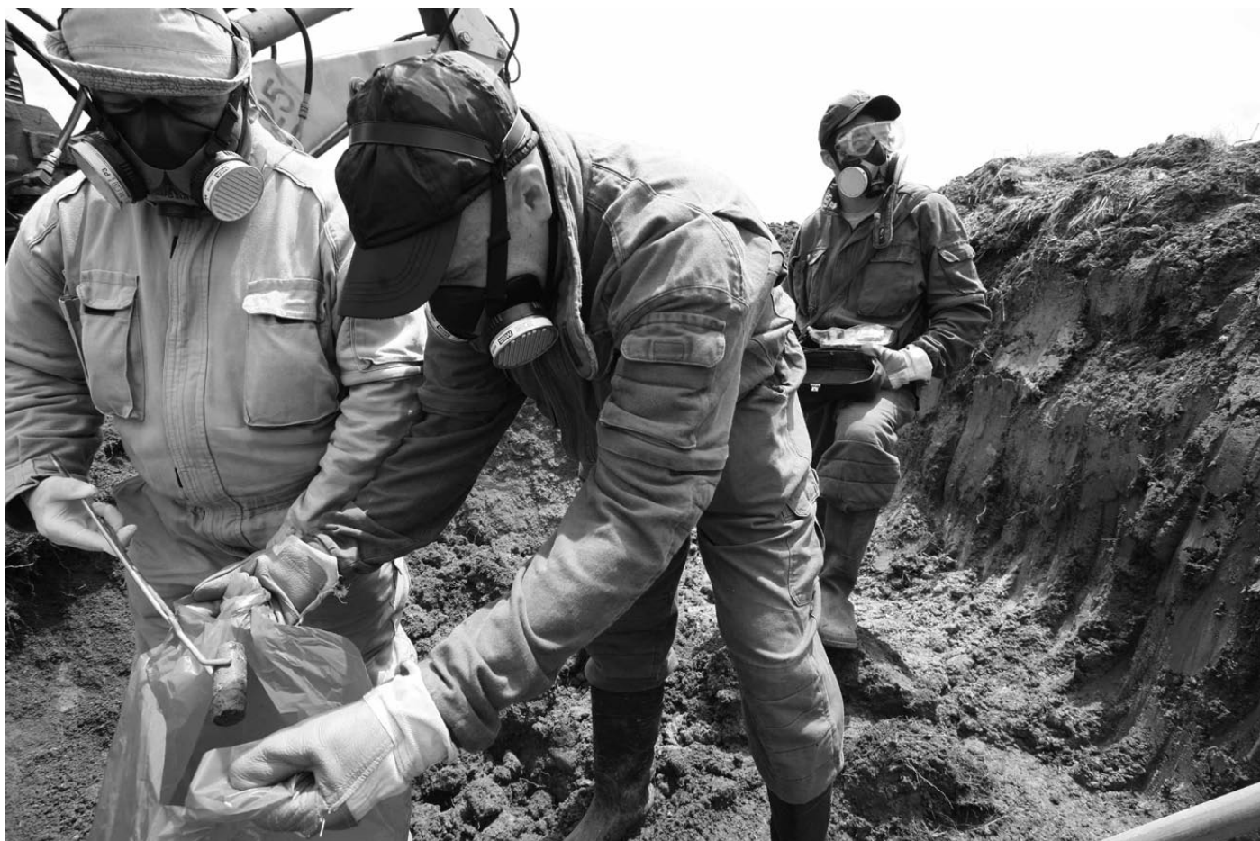
Serbian decontamination team removing the 'jacket' of a 30mm DU round at Borovac in 2007. Contaminated materials and soil from the site were removed to the Vinca Nuclear Institute near Belgrade for vacuum packing and indefinite storage in their low-level waste repository.
