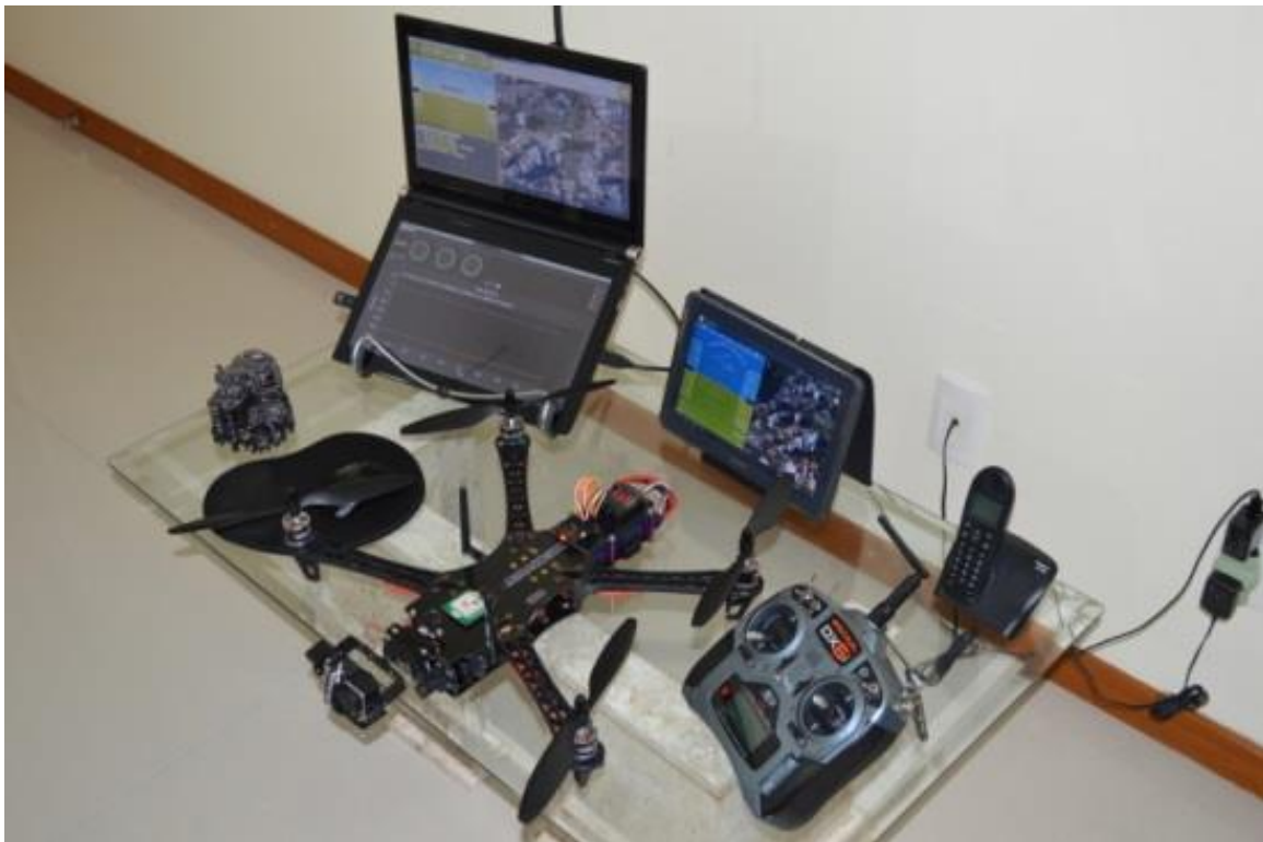
Photo 5: an example of a small UAV ground control station, or GCS (photo credit: Gary McCray)
